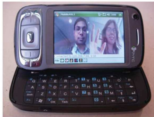
Figure 1. A screen shot of the MobileASL system running on the HTC TyTN-II cell phone. The author and his colleague are shown signing to each other.
